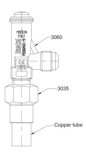
Unions series 3035 allow assembling safety valves series 3030 and 3060 or shut-off valves series 3032, 3033 and 3063 close to the pressure equipments to protect, set up in a refrigerating system.
